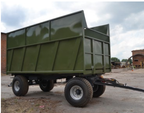
2TSP-14 chip carriers with a body volume of 24 m³
